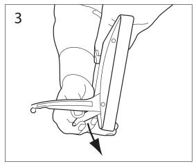
Please follow this step if you require the unit to be positioned behind a keyboard. Un-click leg lifters behind leg, and un-fold them until they click in latch. Ensure both leg lifters are adjusted to the same height.
