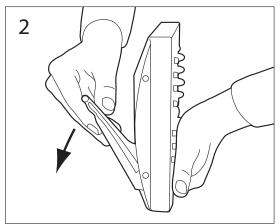
Un-fold legs to desired position. Ensure both legs are adjusted to the same height.
